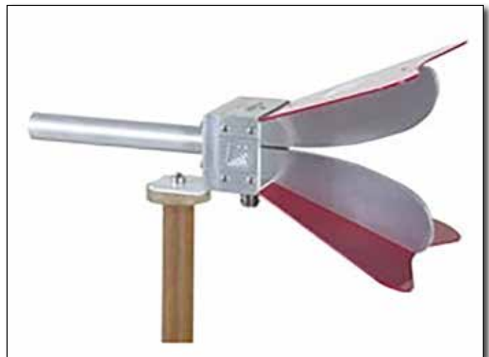
FIGURE 6: Traditional microwave DRG horn as specified in MIL-STD-461E/F and newer version not specified in MIL-STD-461
